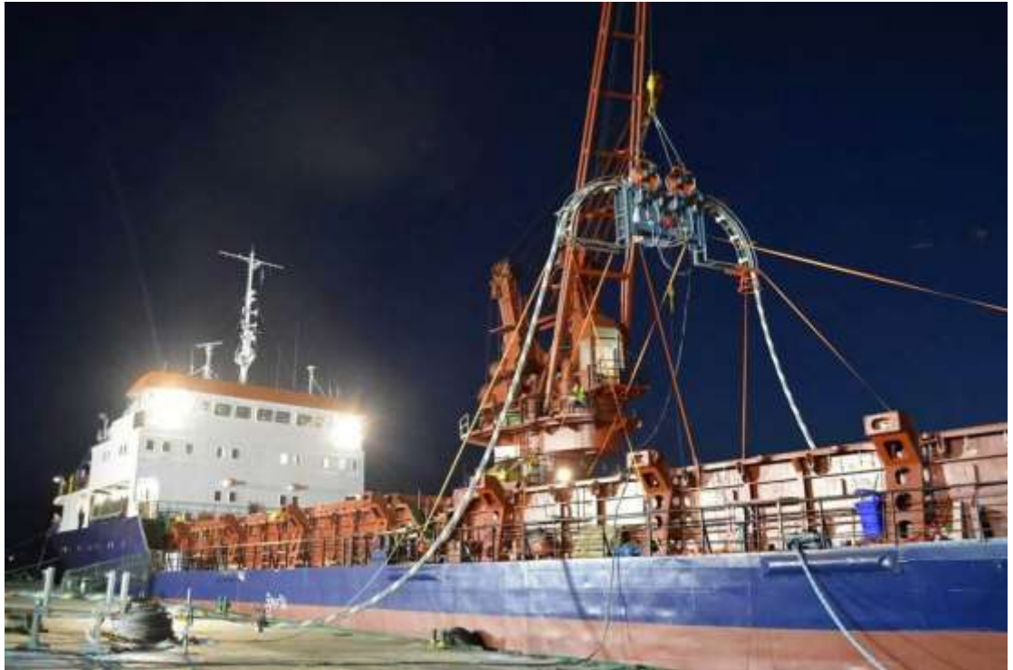
Photograph with Cable Engine on top of the hatch cover
